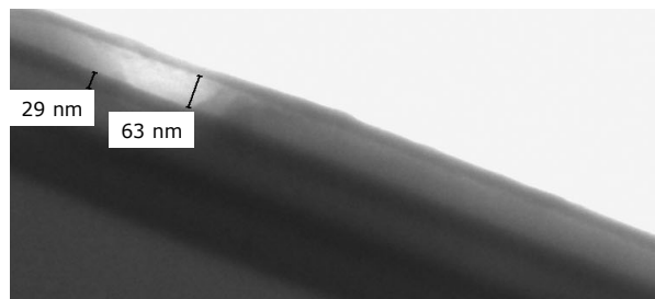
Figure 1. TEM cross-section of the multi-layer structure.
