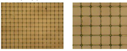
Optical microscopy images on a SIM 1 sample of 50x50 lines, obtained with 2PP. The sample velocity was 1 mm/s. The spacing between the lines is 50 microns and the initiator was IRGACURE 369
