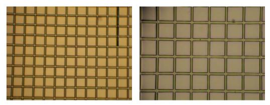
Images on a 20x20 lines SIM 4 sample. The laser power is 5 mW and the sample velocity 0.5 mm/s. The spacing between the lines is 100 microns and the initiator was benzophenone.
